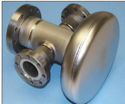
**Figure 3.1 Unmodified BNL 1.3 GHz gun cavity.**
