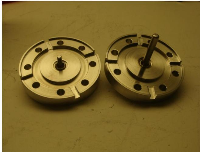
**Figure 3.6 The input coupler and pickup coupler for the gun.**
