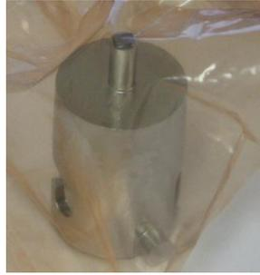
**Figure 3.10 GaAs crystal welded on the plug by indium.**
