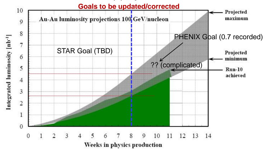
Assume 6 weeks to ramp-up for min, and 8 weeks for max (stoch. cooling re-commissioning). Expect  $L_{\text{avg}}$  up to  $25 \times 10^{26} \text{cm}^{-2} \text{s}^{-1}$  (+25%).
