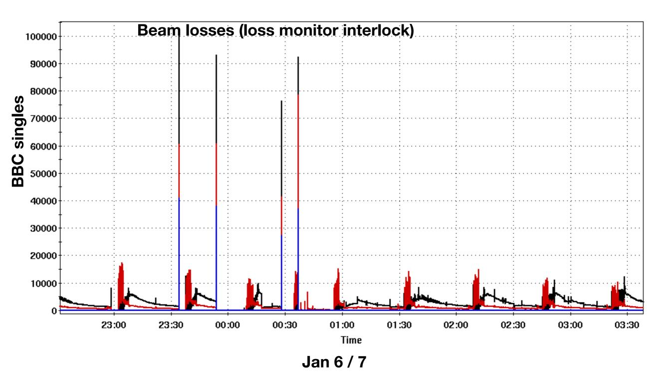
Large backgrounds inducing high and potentially damaging current on the detectors
