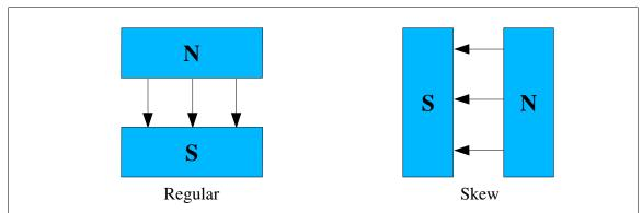
Figure 2: The field directions for the Horizontal (regular) and Vertical (skew) bending dipoles when the magnet is powered with polarity A. Skew dipole: Clockwise rotation of 90°.
