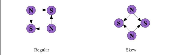
Figure 3: The regular and skew field lines for the quadrupoles in the accumulator ring. These field lines for polarity A. Skew quadrupole: Clockwise rotation of 45°.
