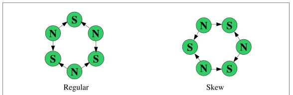
Figure 4: Sextupole field lines for regular and skew magnets. As above, these field lines are for polarity A. Skew sextupole: Clockwise rotation of 30°.
