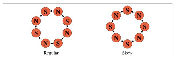
Figure 5: The regular and skew field lines for the octupole correction magnets. These are the field lines for polarity A. Skew octupole: Clockwise rotation of 22.5°.
