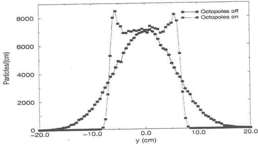
Figure 2.6.4b. Vertical beam profile at target
