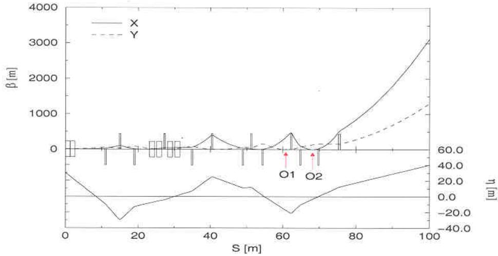
Figure 2.6.2 Optics of the beam transport line.
