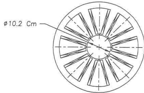
FIGURE 2·7·3 – OCTUPOLE MAGNET
