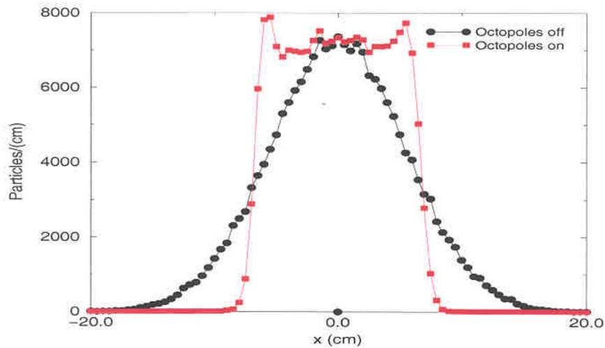
Figure 2.6.4a. Horizontal beam profile at target
