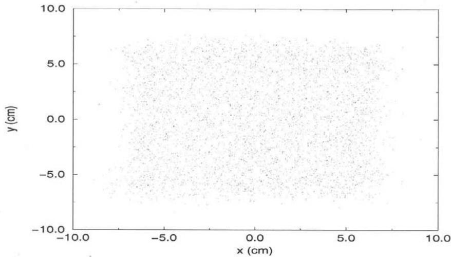
Figure 2.6.5. Beam spot at target.
