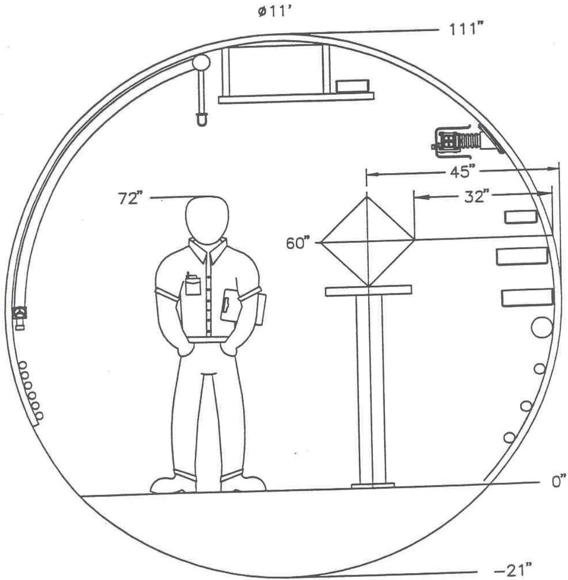
FIGURE - 2.1.4 - TYPICAL TUNNEL CROSS SECTION
