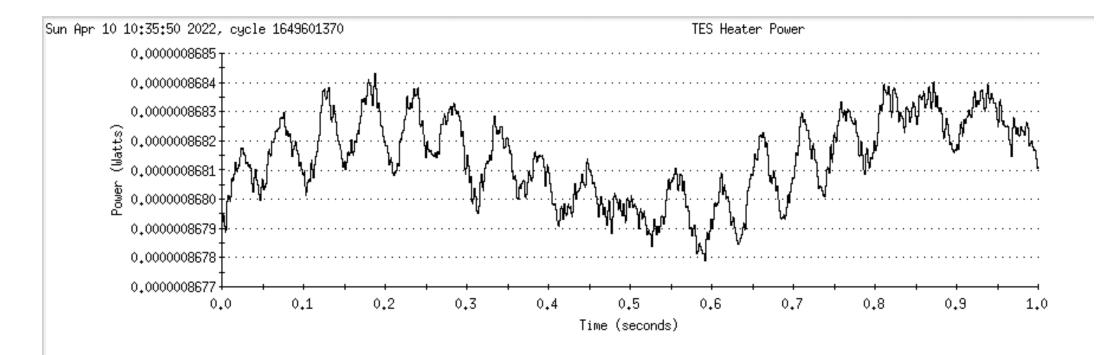
Frequency is about 19 Hz (second harmonic of girder resonance frequency? – sinewave is crossing zero twice). Its level is also much stronger in the beginning of the fill.
