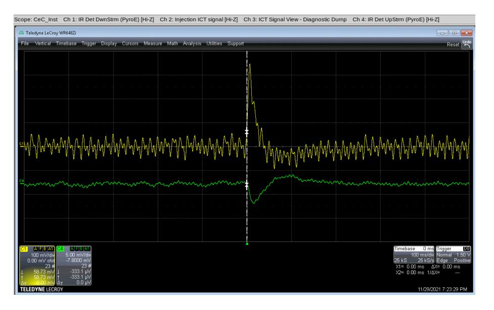
Yellow trace is from downstream pyroelectric detector, green is from upstream pyro.
